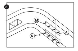
Use type A straight irons to connect the headboard and side rails
