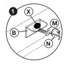
**NOTE**: The type M bolts are not in the hardware kit. They are already pre-installed.
