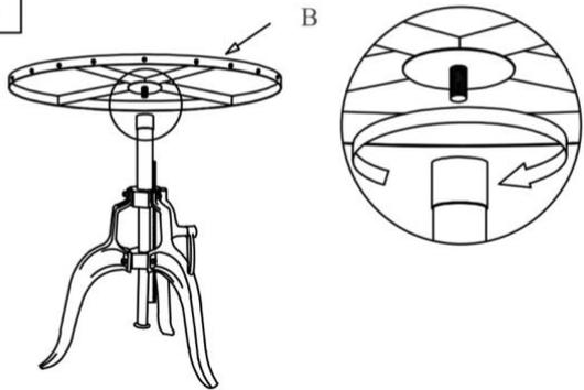
PLACE TOP PLATE C OVER THE BASE & ROTATE CLOCKWISE AND FIX IT WITH THE HELP OF BOLT. ADD TIGHTENER F FOR THE STABILITY OF TOP.
