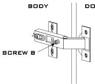
HOW TO FIX IT TO MOVE THE DOOR TOWARDS OR AWAY FROM THE UNIT, ADJUST SCREW "B" AND MOVE THE DOOR FORWARDS OR BACKWARDS UNTIL THERE IS AN EVEN GAP BETWEEN THE DOOR AND THE FRONT EDGE OF THE SIDE PANEL.
