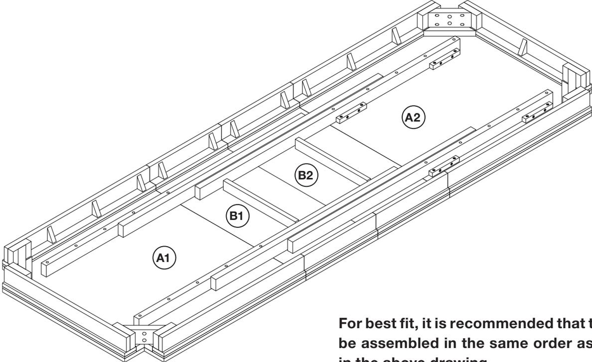
**For best fit, it is recommended that the table be assembled in the same order as labeled in the above drawing.**
