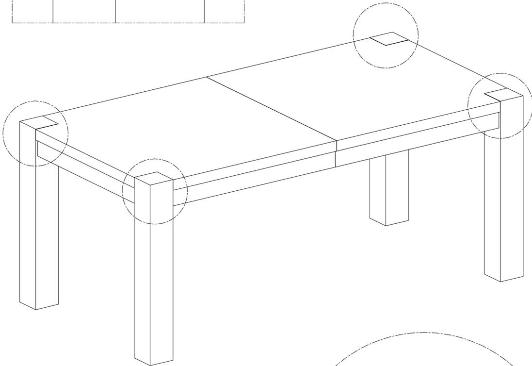
**Rotate the table upright. Align each leg on both sides. Then fully tighten all nuts.**
